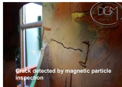
**Crack detected by magnetic particle inspection**
